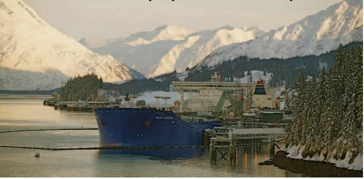
The ConocoPhillips double-hull tanker, the Polar Adventure, transports North Slope crude from Valdez to the Lower 48 and Hawaii. The vessel and other new tankers carrying North Slope crude feature dual independent engine rooms, dual propulsion and steering systems, bow thrusters, and highly sophisticated navigational and control systems.
