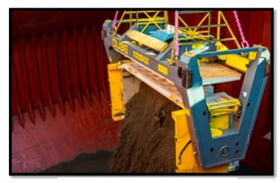
Revolver tipping container in ship's hold
